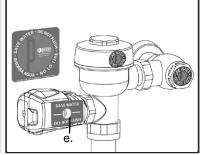
5. Place 'Save Water' velcro (e) back onto IR lens to prevent flushing.
