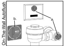
flush valve and the 'Do Not Flush' Sticker (b) on the wall where most visible.
