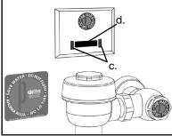
1. Place 'Save Water' decal (a) on the 2. Place 2 Velcro strips (c) on the outside of the AutoFlush lens / infrared sensors (d).
