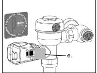
4. To FLUSH, simply remove the 'Save Water' velcro (e).
