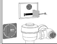
4. To FLUSH, simply remove the 'Save Water' velcro (e).
