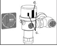
outside of the AutoFlush lens / infrared sensors (d).
