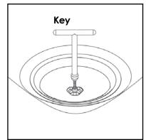
2. PUSH then screw the Threaded Key into the center hole.
