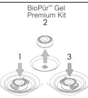
Push Down on edges of BioPūr<sup>™</sup> Kit cover and Turn counterclockwise to remove the BioPūr<sup>™</sup> Kit (#1). Recycle the used BioPūr<sup>™</sup> Kit (#2). After removing protective packaging, screw a new BioPūr<sup>™</sup> Kit onto EnviroSeal<sup>™</sup>. Turn clockwise until firmly in place, DO NOT OVERTIGHTEN (#3).
