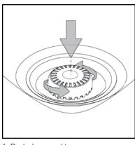
Push down and turn counterclockwise to remove the BioPūr<sup>™</sup> Kit or Privacy Dome from the EnviroSeal<sup>™</sup>. Please recycle.
