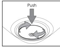
4. Firmly push down around ENTIRE CIRCUMFERENCE of EnviroSeal<sup>™</sup> outer edge to ensure it is in place with NO gaps between Enviroseal<sup>™</sup> and metal ring.
