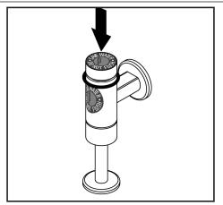
3. To flush the urinal, remove the O-ring from the groove, then push.
