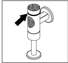
4. Place the O-ring into groove when completed.
