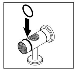
2. Place the industrial grade strength Pūrleve O-Ring in the groove between Push Button and valve.
