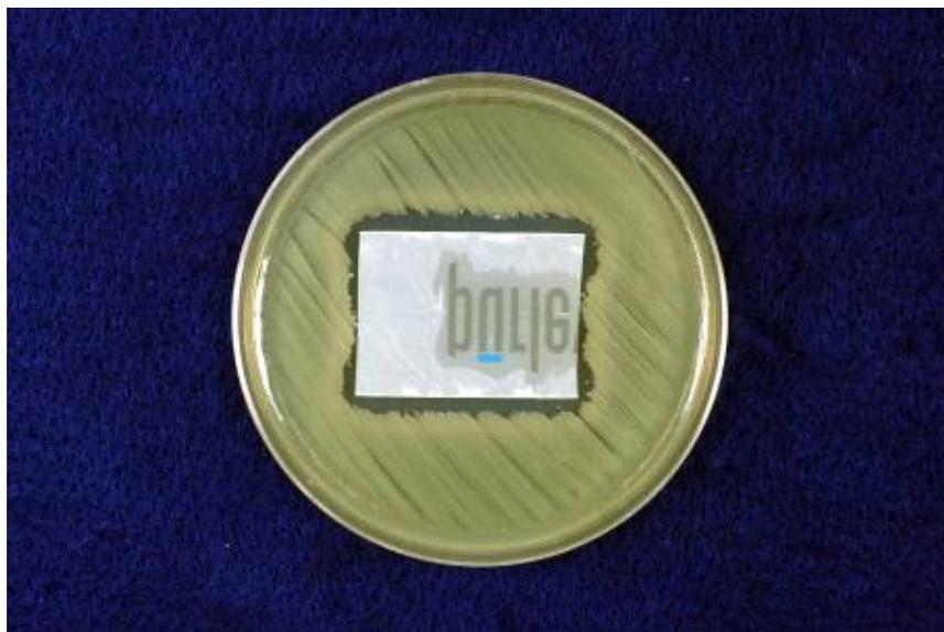
Treated Sleeve Sample Replicate 2: the film is exerting an antimicrobial effect against the bacteria. Note there is an area of inhibition around the sample where the growth of the bacteria has been effectively suppressed.
