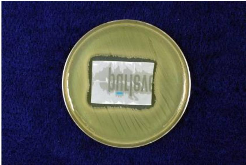
Treated Sleeve Sample Replicate 1: the film is exerting an antimicrobial effect against the bacteria. Note there is an area of inhibition around the sample where the growth of the bacteria has been effectively suppressed.
