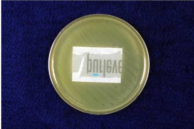
Control Sleeve Sample: the *E. coli* bacteria has grown all the way to the edge of the sample and is also found underneath the sample (can't see this from the photo- the microbiologist has to lift the film to examine the agar bed under the sample). This shows that an untreated sleeve film is unable to inhibit the growth of bacteria.
