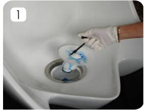
Screw the key into one of the holes of the Drain Insert and pull upward to remove. When insert is pulled, the contents of the waste trap empties into the waste line.
